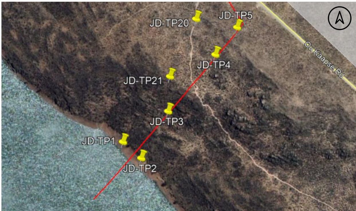
Figure 10: Test pit positions along Rising Main 1
