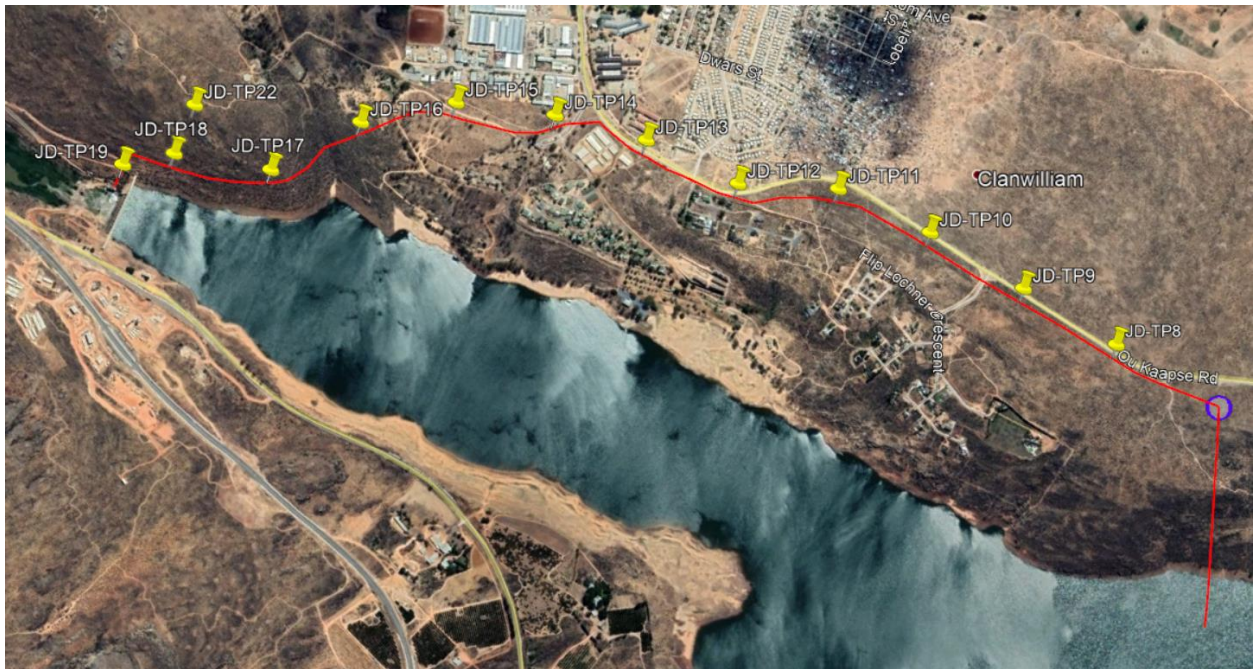
Figure 11: Test pit positions along Rising Main 2
